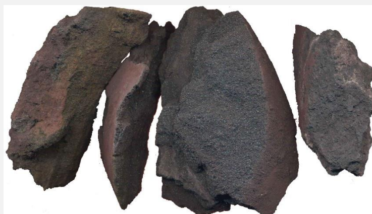
Figure 7. A color photograph illustrating the general nature and appearance of this sample in hand specimen. Note the sugary texture exhibited by the core, largely due to the porous and granular nature of the martite. The width of view is approximately 10 cm.
