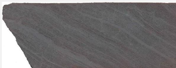
Figure 9. A color photograph illustrating the general nature and appearance of this sample in hand specimen. The delicate layering appears to reflect, in part, significant variations in porosity. The less porous hematite may also cross-cut the more porous laminations. The width of view is approximately 11 cm.
