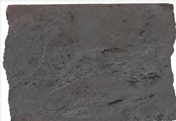
Figure 14. A color photograph illustrating the general nature and appearance of this sample in hand specimen. This laminated sample exhibits a somewhat fragmented appearance with a wide variation in porosity. The width of view is approximately 9 cm.
