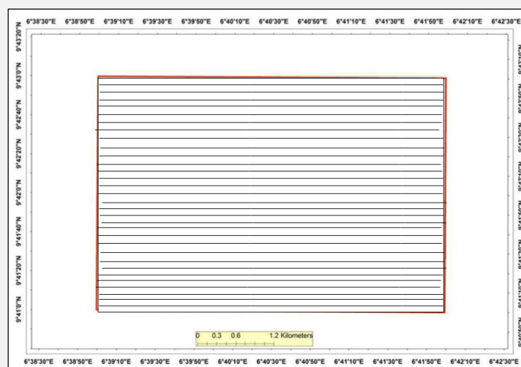
Figure 3. Profile lines of ground magnetic surveyed area.
